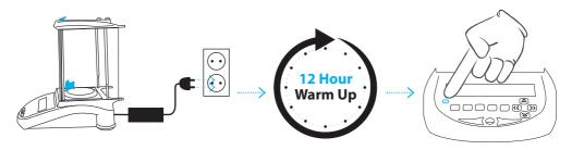
The balance must be plugged into the mains power and turned on for a minimum of 12 hours, prior to any calibration and use. The balance should then be calibrated before use.
